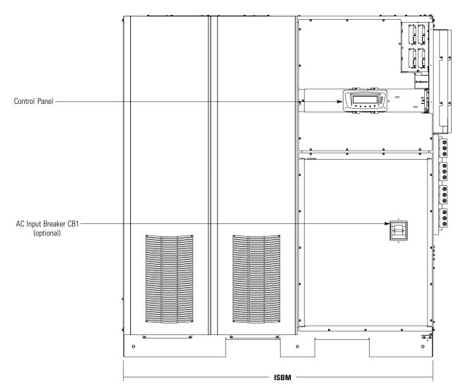
Figure 7-1. UPS Controls and Indicators – ISBM Section Shown
